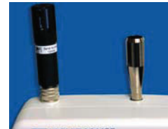
Removable Temp / RH and Isokinetic Probes
